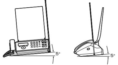
The diagram shows two views of the device. The left view shows the device tilted at an angle, with a 5-degree angle line indicating the maximum allowed tilt. The right view shows the device upright, also with a 5-degree angle line indicating the maximum allowed tilt.
